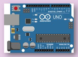
The Arduino Uno is an open-source microcontroller board based on the Microchip ATmega328P microcontroller and developed by Arduino.cc. The board is equipped with sets of digital and analog input/output pins that can be
